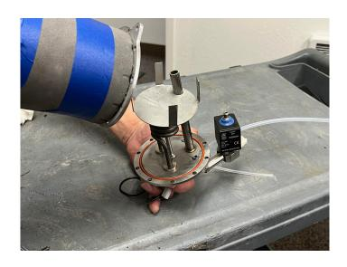
Including the Heating Disk orientated as shown is essential to proper function.
