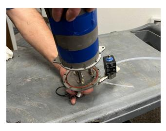
To keep the Heating Disk and main o ring in place, we hold the top plate upside down and slip the shell on as shown.
