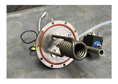
The reassembled top. Note the orientation of the heating element vs the temp probe in the center. It won't fit properly if the heating element is reversed.
