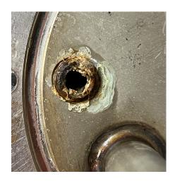
Remove the temp probe, heating element, and any fittings you are going to replace. Examine the inner side of fittings — they can become clogged with hard water scale.
